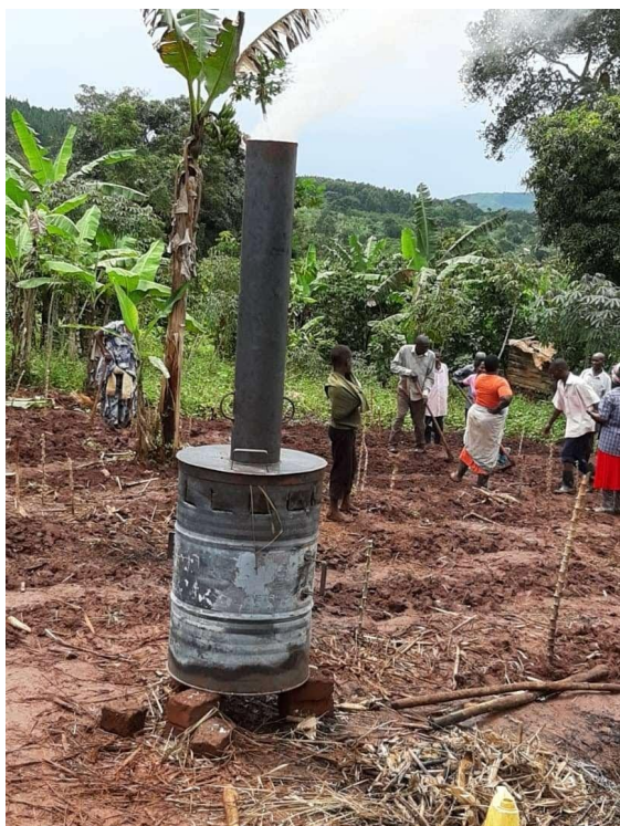
Modified barrel kiln positioned in the field for coffee husk conversion.
