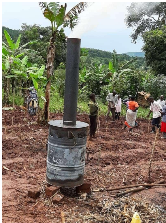
Modified barrel kiln used to convert coffee husks into biochar under field conditions.
