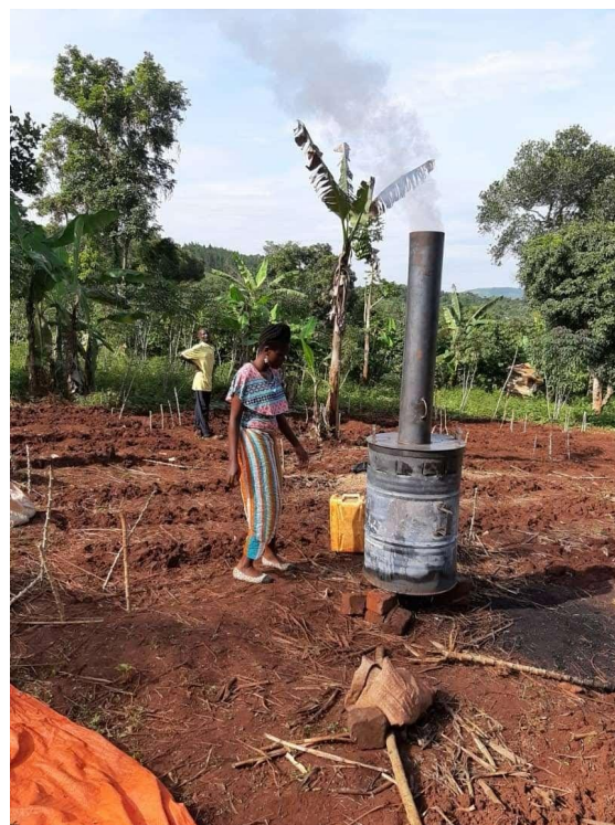
Field operation of the modified barrel kiln during biochar production.
